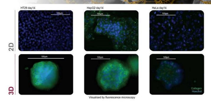
After the 14th day of growth there is significantly more collagen type I (in green) produced in cells grown in 3D for the three cell types tested.
